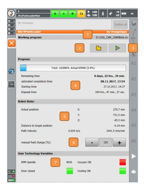
Name and Path of actual CAD/CAM file Button to open the File-Open-dialog. Only active if no program is running Button to load the selected CAD/Cam file into the memory. Only active if no program is running The progress bar shows the number of commands of the CAD/CAM file and the number of the current command. While loading a CAD/CAM file, the loading progress is displayed. More information: Starting time Elapsed time since start
